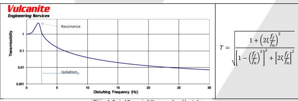
Figure 2: Typical Transmissibility curve of a rubber isolator
