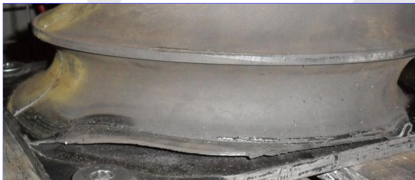
Figure 7: Failure of bond between rubber and metal
