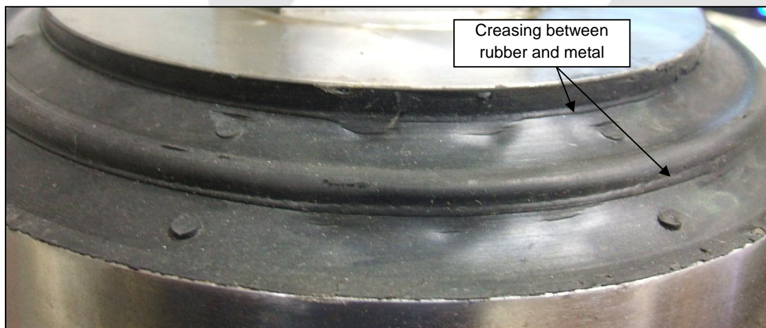
Figure 2: Rubber creasing in a bush after 200,000 km service
